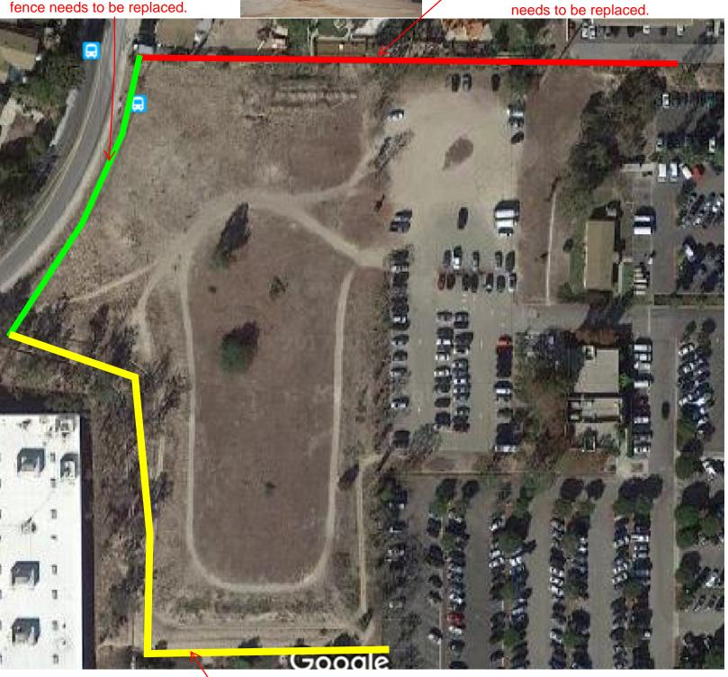
New 8' fence with approximately top 2' slanted -away from the TCMC property. Example of the slant shown in the picture above.
