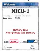
Charge battery by placing into docking station, Takes 2 hours to fully charge battery. Or change battery. Extra battery is stored in docking station.
