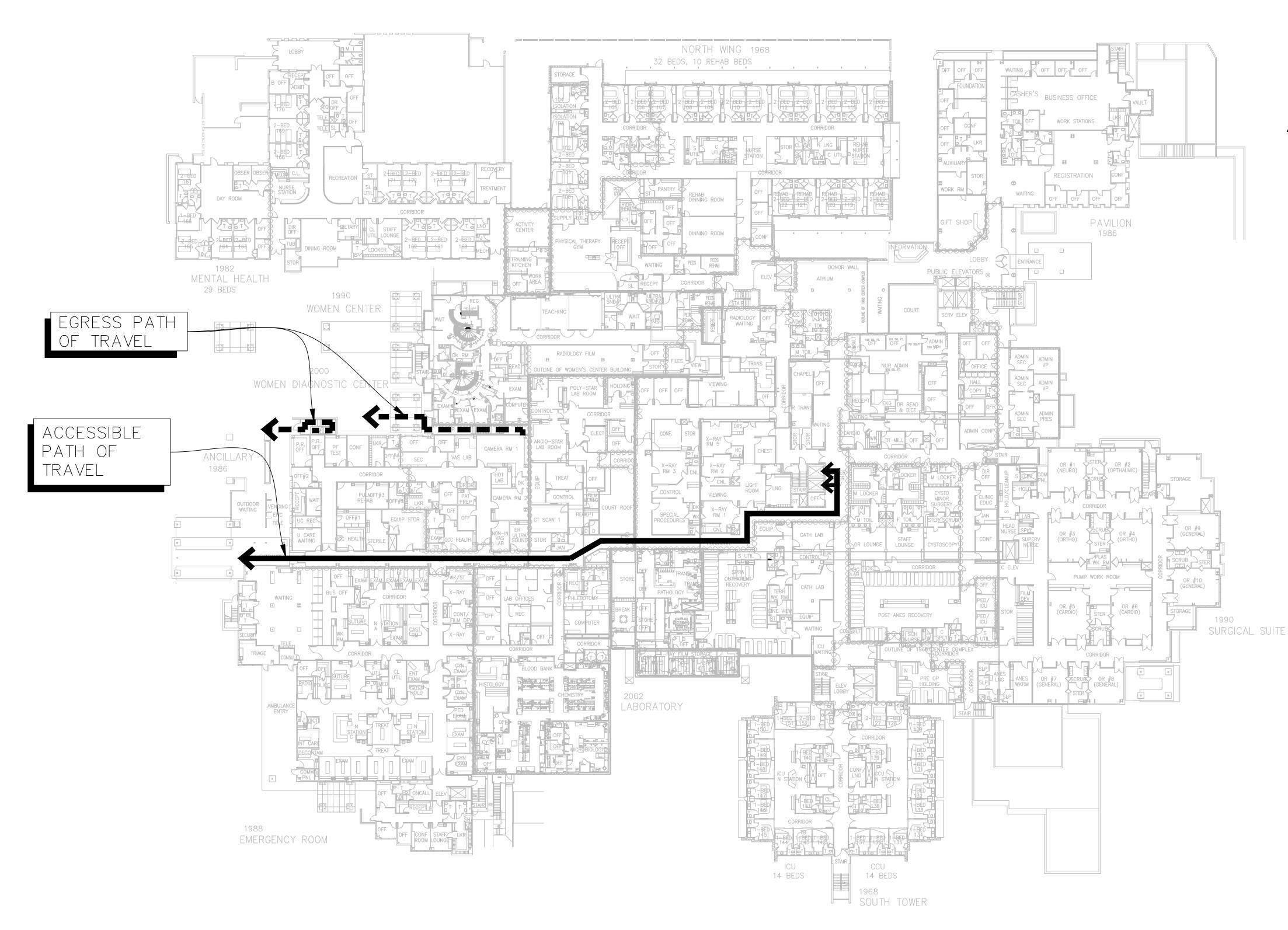
CODE COMPLIANCE FIRST FLOOR PLAN SCALE: 1/32" : 1'-0"
